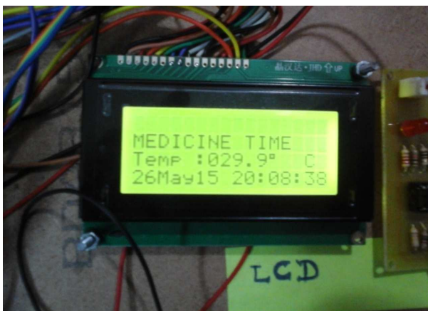
Fig. 8. Medicine Time and Body Temperature of Patient Indicated on LCD.
